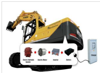
• 21-ton Battery-powered Excavator
